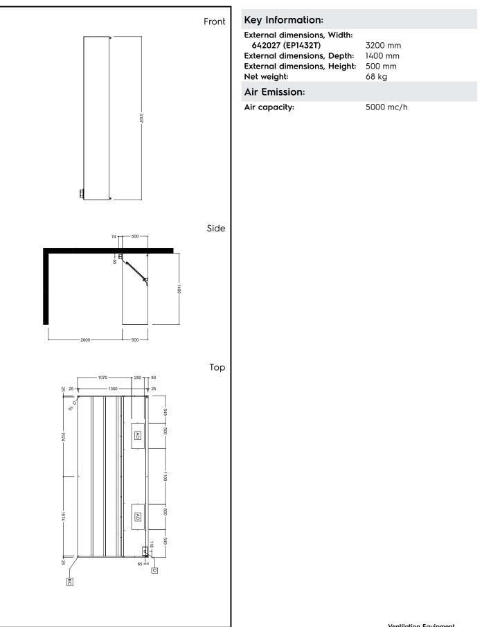
Ventilation Equipment 304 S/S Wall Hood+Filters 3200X1400mm
